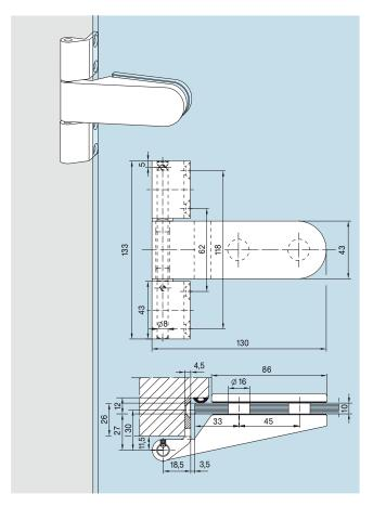
Strengthened hinge with frame pivot for wooden frames, hinge flap for mortising into frame, stainless steel pin, door weight max. 45 kg Art. No. 10.239 Weight in kg: alumin. 0.433
