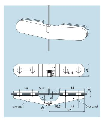
Hinge for mounting onto sidelight, stainless steel pin, door weight max. 35 kg Art. No. 10.245 L (as illustr.) Art. No. 10.247 R Weight in kg: alumin. 0.557
