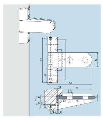
Strengthened hinge with frame pivot for wooden frames,
