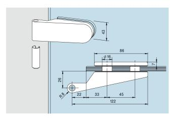
Hinge with frame pivot, complete with sleeve, rebate depth 26 mm, extended colour options, door weight max. 45 kg Art. No. 10.236
