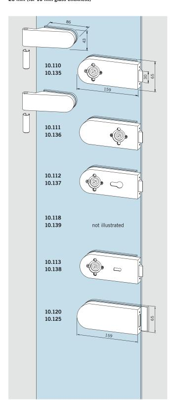
Lock with 2 hinges, non-locking lock, hinges with sleeves 8 mm glass thickness
