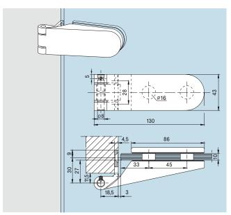
Hinge with frame pivot for wooden frames,
