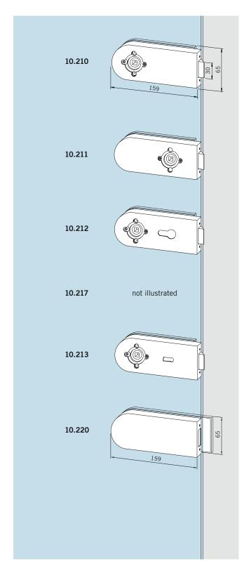
Art. No. 10.210 non-locking, extended colour Weight in kg: alumin. 1.580
