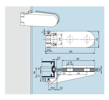
Hinge with frame pivot for aluminium frames, stainless steel pin, door weight max. 35 kg
