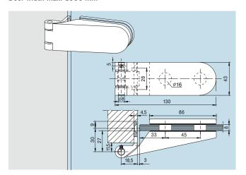
Hinge with frame pivot for wooden frames,
