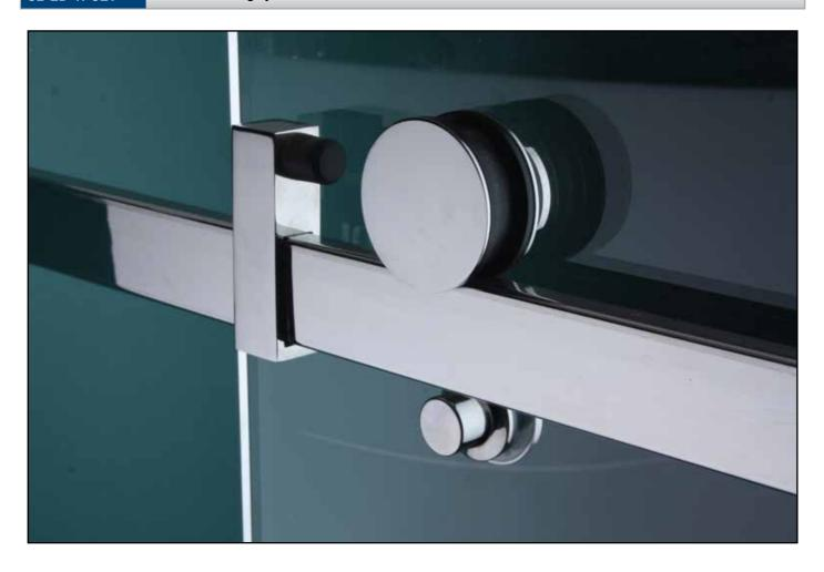
Edge Line sliding system is a self supporting sliding system for in line & 90° doors. Recomended for installation shower cubicles, this system supports the track on the fixed glass itself. A shower threshold is available to ensure 100% water tightness even below the sliding doorway. Standard sets are available for 1.65mtr & 2mtr opening.
