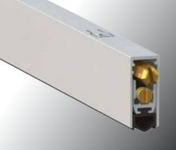
The PRESSURE SERIES is caracterised by the Comaglio twin adjusting mechanism; It is a patented mechanism designed to perfectly close the gap between doors and floors. The downward pressure applied by the seal to the floor is equal across the full width of the door. This is essential for optimal sealing in normal conditions and particularly important in more difficult situations such as uneven floors, tilina etc...
