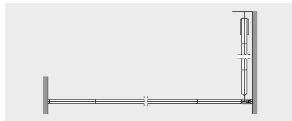
Parking solution PLD – Two-point suspension – 90° to partition axis – Parked in a row arrangement
